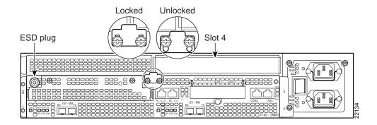
Depending on your circumstances, you might need to install a new port adapter in a Cisco 7100 series router or replace a failed port adapter in the field. All port adapters available for the Cisco 7100 series connect directly to the router and are locked into position by a locking tab with two screws (see Figure 7-1 or Figure 7-2). You need a number 2 Phillips screwdriver to loosen the screws.
